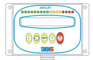
• *Emergency stop pushbutton*: when pressed down, it cuts out power to the electric motors and blocks the movements of the machine.
