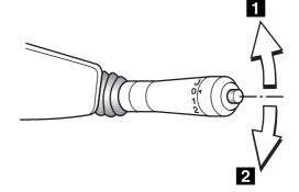
Set lever to pos. 1 to indicate a turn leftwards or to
